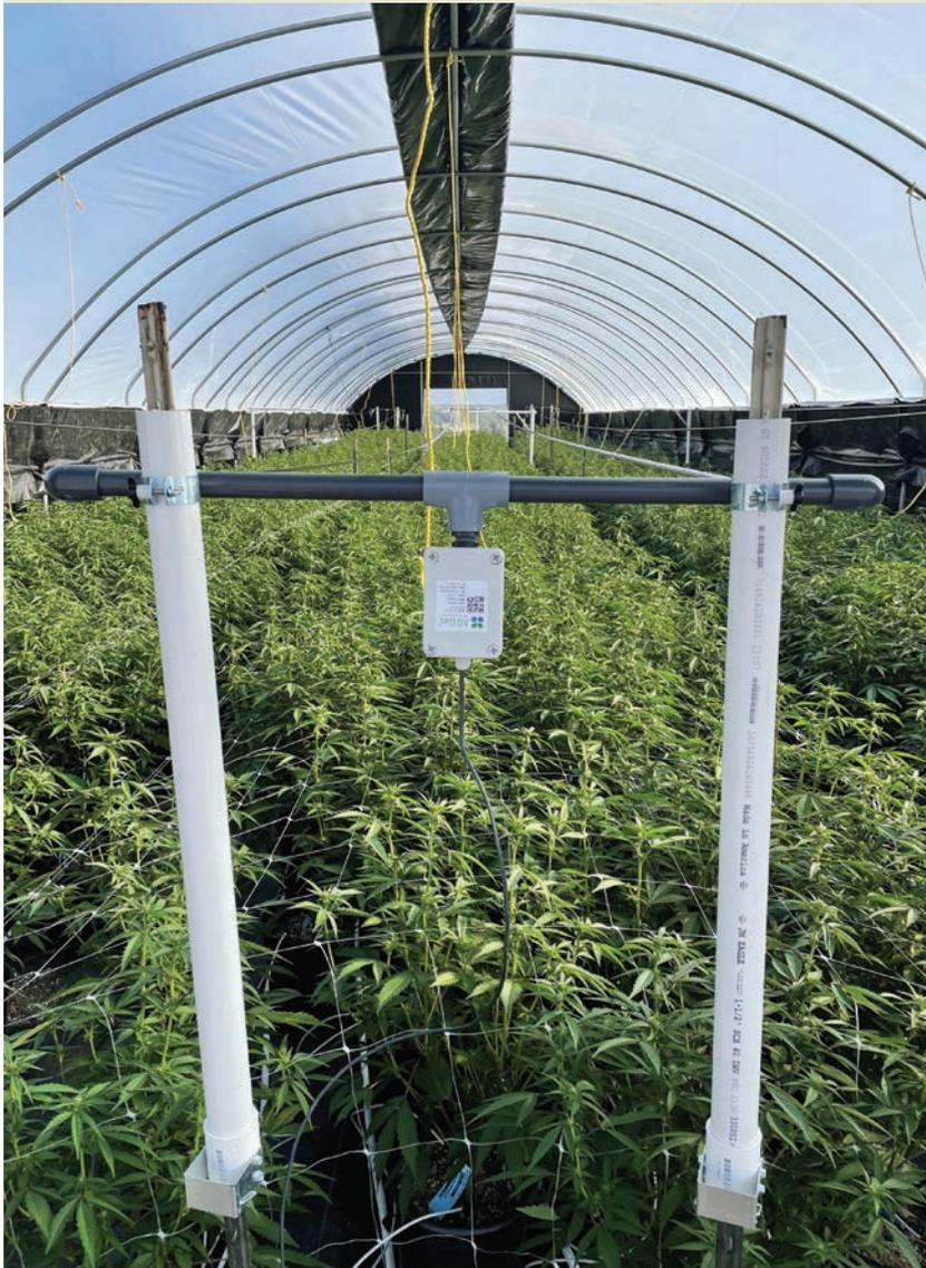
The Carbocation black box control unit adjusts gas flow in real-time to deliver optimum results based on extant field conditions. The unique configuration allows for prescriptive delivery of CO<sub>2</sub> gas to the plants. Photo: AgGas
